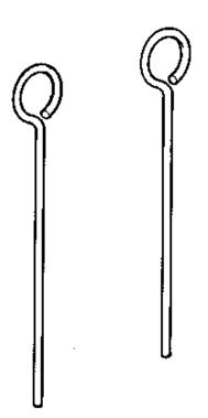
Note: For locking chain tensioner piston in position
