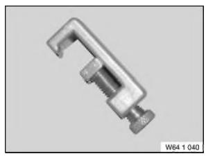
Note: Aid to fitting drive belt (power steering pump
