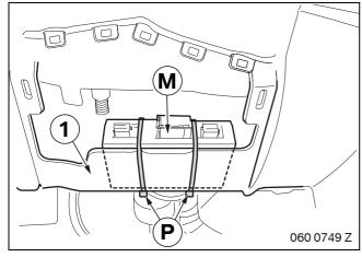
Secure the LVDS converter **M** to the trim (1) below the steering column using cable ties **P**.
