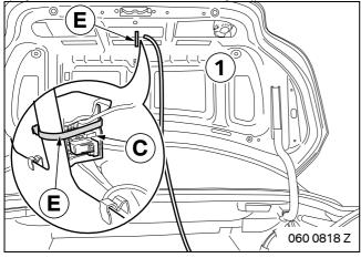
Use cable tie  ${\bf E}$  to attach control unit  ${\bf C}$  to the web of the boot-lid (1).
