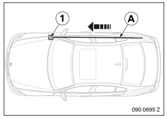
Route Rear View wiring harness **A** along the standard wiring harness into the footwell on the passenger side (1).
