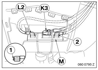
Use the coding (1) on the plugs to connect them correctly. ◀
