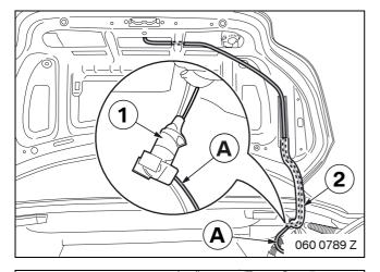
Route rear view wiring harness **A** through the hinge tube (2) and cable grommet (1) into the boot.
