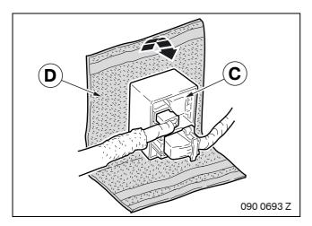
Affix protective strip **D** to control unit **C**. Cut off any excess lengths.
