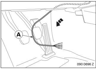
Route Rear View wiring harness **A** along the standard wiring harness into the footwell on the driver's side.
