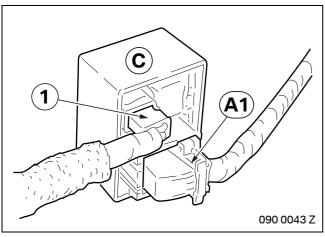
Connect the connection plug (1) of the rear view and branch **A1** (12-pin black plug) to control unit **C**.
