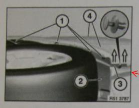
Release screws (1) from wheel arch cover (2) on left/right. Release expansion rivet on left/right.
