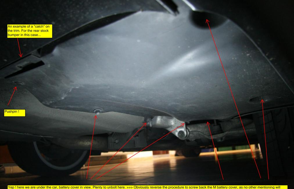
Yep! here we are under the car, battery cover in view. Plenty to unbolt here. >>> Obviously reverse the procedure to screw back the M battery cover, as no other mentioning will take place on this straightforward item!
