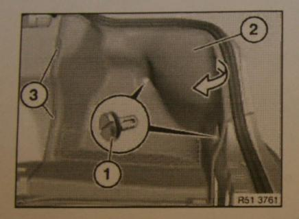
Open rotary clips (1) and remove.
