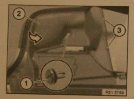
Open rotary clips (1) and remove.
