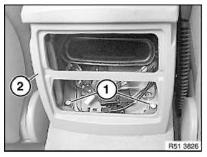
Release screws (1) on storage tray at rear. If necessary, unlock plug connections.
