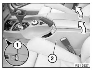
Release handbrake lever gaiter on storage tray (2).
