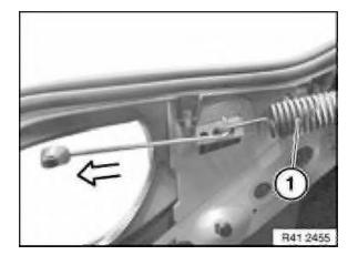
Attach special tool 51 3 290 in tension spring (1) and pull towards rear.
