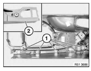
Release screws (1) on inside of storage compartment and remove trim (2).
