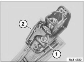
Release screw (1) and remove fastener (2).
