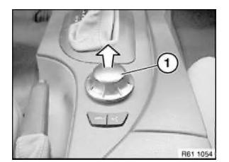
Detach knob for controller (1) in direction of arrow.
