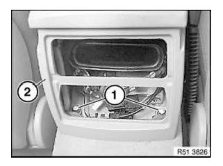
Release screws (1) on storage compartment (2). If necessary, unlock plug connections.
