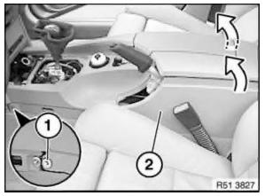
Release handbrake lever gaiter on storage compartment (2).
