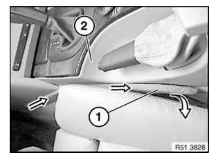
Lever out trims (1) on left/right at rear end and pull out in direction of arrow.
