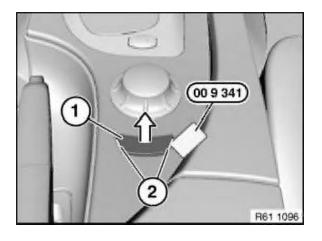
Unclip button unit (1) with special tool 00 9 341 at retaining points (2) and lever out in direction of arrow.
