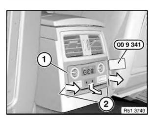
Unclip rear insert (1) with special tool 00 9 341 at retaining points (2) and pull back in direction of arrow. Disconnect associated plug connections and remove rear insert (1).
