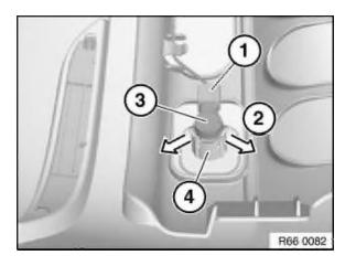
Unfasten plug connection (1) and disconnect. Unlock catches (2) in direction of arrow and pull ultrasonic transducer (3) out of bracket (4).
