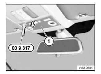
Lever out ceiling light (1) with special tool 00 9 317 as illustrated.
