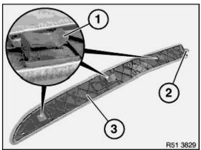
Release handbrake lever gaiter on storage tray (2).
