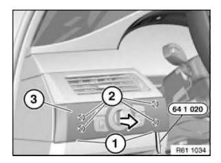
Attach special tool 64 1 020 at openings (1) and lever out catches (2). Pull back lighting control unit (3).
