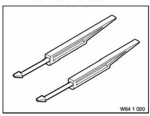
Note: For releasing and removing fresh-air grills - For
