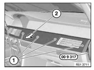
Lever out right decorative strip on instrument panel (2) at retaining points (1) with special tool 00 9 317 .
