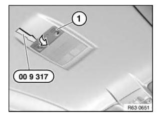
Lever out ceiling light (1) with special tool 00 9 317 as illustrated. Disconnect plug connection underneath and remove ceiling light (1).
