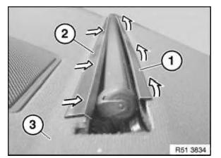
Lift out shelf (3) over rear groove (1) of rear window roller blind. Pull front guide (2) out of shelf (3) and remove roller sun blind towards bottom.
