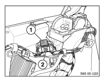
8. Locate fiber optic distribution block (1) and unscrew 10mm Hex nut (2).
