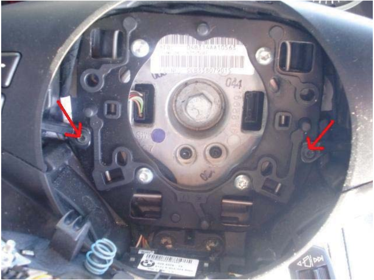
Once these are done up all you have to do is push the airbag back in & you will hear it clip in & you are now done.
