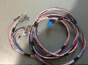
I have used 12 wires with 0.5mm2 (16x0.2) with length about 2.5 meters and I have had about 20 cm left as spare, hidden behind the panel.
