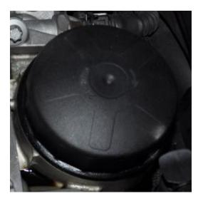
I reused my old filter and cap o-ring because I will change the oil in the next month. There is a risk of creating another leak at the cap by reusing this. However, I did not get a leak. Just make sure to clean well and lubricate with oil on the ring and inside the housing
