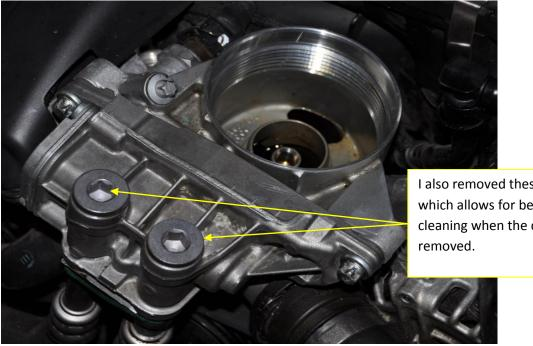
I also removed these two caps which allows for better cleaning when the cover is
