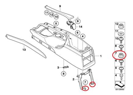
Mine had an additional plug with wires connected to the back (I believe it was for the cell phone cradle). It's held on by a plastic clip and small torx screw at the base of the center of the rear part of the console. Lift console up and remove the torx screw if you have this.
