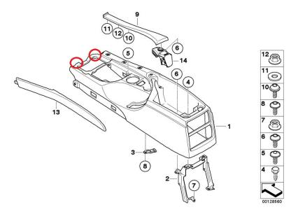
7. Slide carpet covers on each side of the console (#13) toward the back of the car. This will expose 2 screws securing the sides of the console.
