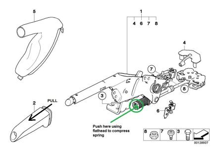
13. Once that spring is compressed, you can raise the handbrake handle all the way up – enough to allow you to remove the console. This was my **AH-HA!** moment.
