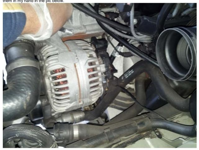
12. Once the bolts of the alternator are removed, the trick to remove the alternator is to give it a good jerk as if you are trying to lift it out.
