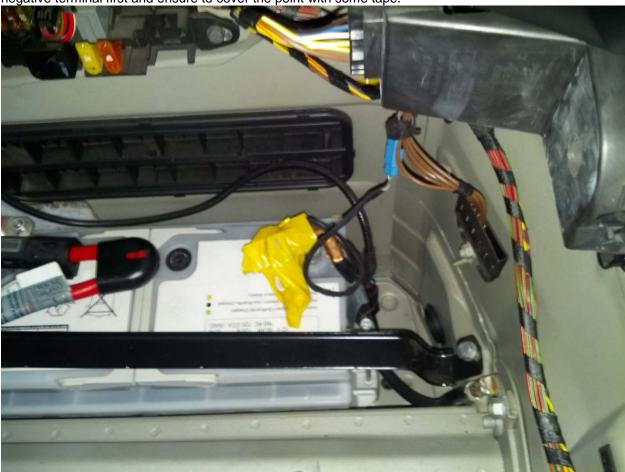
7. The positive terminal can be dis-connected after the negative one, but is not necessary. So you decide for yourself. I won't have any negative impact anyways IMHO.
