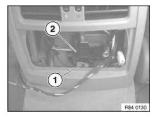
If necessary, unlock antenna connector (1) and disconnect.
