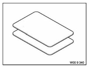
Note: For levering out switch pad on driver's door
