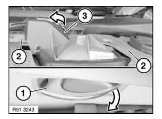
Unhook Bowden cable for release lever:
