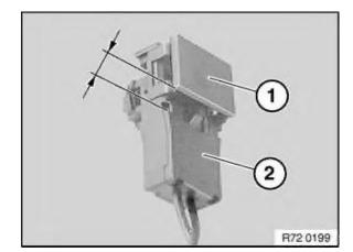
Cover (1) is not positioned higher than housing (2). The airbag plug connection is unlocked and can now be detached from the gas generator/airbag module.
