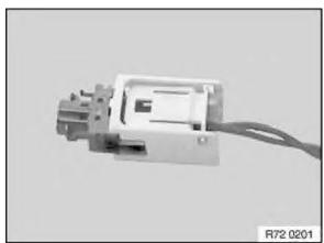
The airbag plug connection is unlocked and can now be detached from the gas generator/airbag module.
