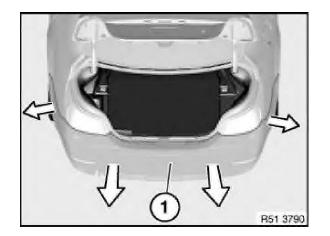
Unclip bumper trim (1) to side panel (1) on left/right outwards. Remove bumper trim (1) in direction of arrow towards rear. With optional extra PDC:
