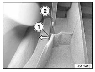
Unclip pin (1) from shock absorber (2).
