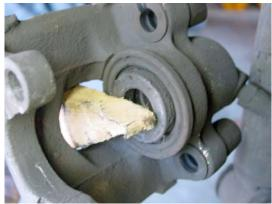
This is because the new pads are going to be quite a bit thicker than the old ones, and the piston is set in the old pad so position. Pry back the piston using the wood, being careful not to use too much force. Using a screwdriver here can accidentally damage the dust boot and seals inside the caliper, and is not recommended.
