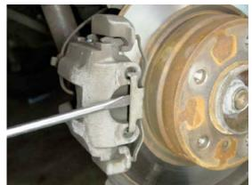
Make sure you wear safety glasses during this step, as the clip can come flying off if you're not careful. Then, use a pair of needle-nose pliers to remove the brake pad sensor
