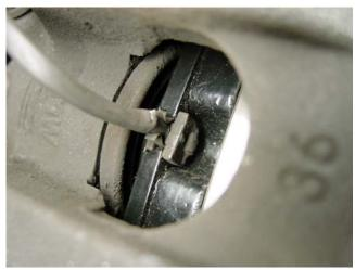
You also may want to spray the back of the brake pads with some anti-squeal glue. This glue basically keeps the pads and the pistons glued together, and prevents noisy vibration. Anti-squeal pads can also be purchased as sheets that are peeled off and placed on the rear of the pads.
