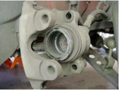
Once you have the pads removed, inspect the inside of the caliper. You should clean this area with some compressed air and isopropyl alcohol. Make sure that the dust boots and the clamping rings inside the caliper are not ripped or damaged. If they are, then the caliper may need to be rebuilt.
