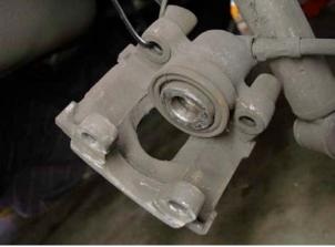
Suspend the caliper using some zip-ties or rope - don't let the caliper hang from its rubber hose (very bad). See Figure 8
