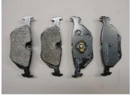
into the caliper. If you encounter resistance, double check to make sure that the inside of the caliper is clean. Simply snap the inner brake pad into place using your hand (Figure 12).
