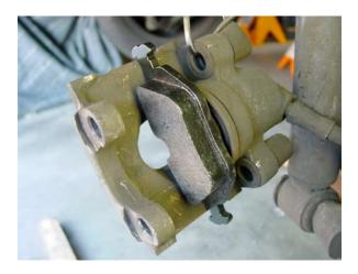
The process for assembly is the reverse of the disassembly. Mount the caliper back onto its mounting bracket, surrounding the brake disc. If the caliper won't fit, then you need to push in the piston a bit more until the space in-between both pads is wide enough for the brake disc to fit. Tighten down the guide bolt using a torque wrench to 22 ft-lb (30 Nm).
