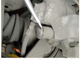
The BMW caliper used on the 3-Series (and many other BMWs) is a single piston caliper design. One piston presses against the side of the brake disc, and the whole caliper slides on the guide bolt to achieve equal pressure on the disc from both pads.
