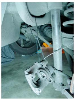
for details. As this point, you can pluck the outer brake pad out of the caliper, and use a screwdriver to pry the inner pad out of the caliper piston. The caliper should resemble Figure 9 when you're done.
