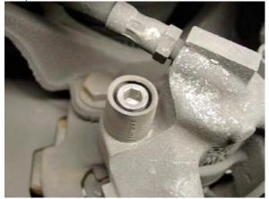
with a 7mm allen wrench (thanks to Barney McComas for the tip). Then remove the brake pad retaining clip (keeps the pads from rattling), shown in Figure 5.
