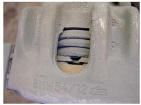
Begin by removing the small plastic cap that covers the caliper guide bolts (Figure 3).
