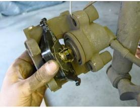
When firmly mounted, the new pad should resemble Figure 13.
