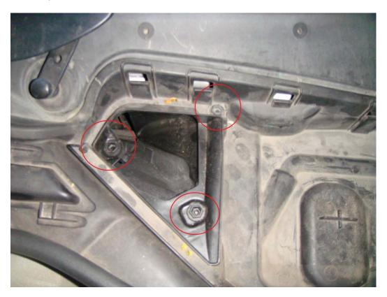
8. Pull up clip and slide towards drivers side then lift up and remove plastic piece.
