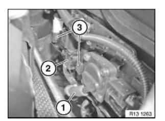
Pull off hose (1). Unlock plug connection (2) and remove. Unlock connector (2) and remove. Unlock plug (3) and remove.
