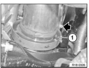
Release screw. Tightening torque 18 32 1AZ . Remove V-clamp (1).
