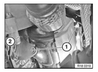
Release screws (1). Unfasten screws (2). Remove diesel particulate filter.
