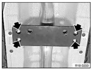
Unfasten screws. Remove reinforcement plate. Lower exhaust system carefully.
