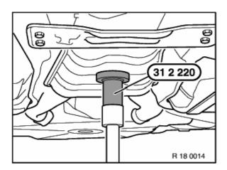
Support exhaust system with special tool 31 2 220 .
