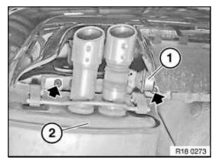
If fitted: Pull off vacuum hose (1). Unscrew nuts (1).
