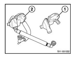
1. Replace the oil separator and hoses (1) with the new insulated style (2).
