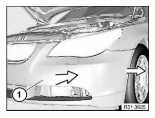
Press bumper trim (1) against direction of travel and release from holders in direction of arrow.
