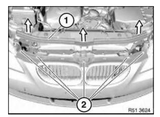
Unclip strip (1) in direction of arrow and release screws (2) underneath.
