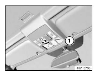
Unclip front roofliner trim (1) in direction of arrow.
