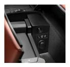
To allow the use of the audioplayer function of a mobile phone inside the vehicle via the USB interface, the BMW Group offers the USB audio interface\* (option code **6FL)** for current BMW new vehicles (excluding X3). For
