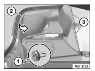
Open rotary clips (1) and remove.
