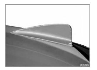
The GSM antenna is integrated into the telephone and GPS aerial. The telephone and GPS aerial is installed on the rear edge of the roof.
