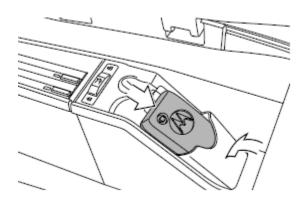
The Bluetooth® Upgrade Module (BTUM) is shaped exactly like a CPT9000 (Motorola V60 series) phone and is installed into the phone cradle in place of the original CPT9000 handset. It provides the link between an approved Bluetooth® phone and the vehicle's original phone system. Up to 2 different phones can be paired with the BTUM; however, only one can be used with the system at a time.
