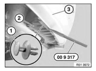
Release expander rivet (1) on guide (2).
