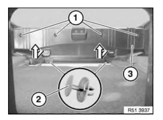
Release protective caps (1) and screws underneath.
