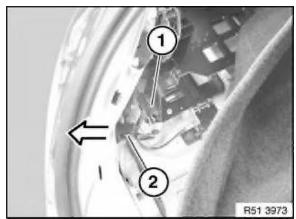
Disconnect plug connection (1) and feed out wiring harness with cable grommet (2) in direction of arrow.
