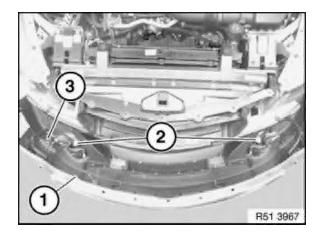
If necessary, disconnect plug connections on fog lamps (2) and/or Park
