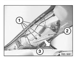
Unlock plug connections (1) and disconnect. Release screws (2). Remove antenna amplifier (3) in direction of arrow.
