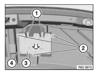
Unlock plug connections (1) and disconnect.
