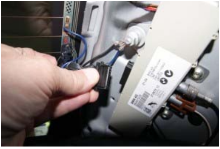
Window harness removed.
