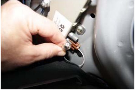
4) Disconnect the antenna output and power connector plugs from the amplifier.
