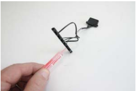
5) Apply the DeoxIT drops to each terminal connection on both ends of the window harness and each of the antenna and power terminals.
