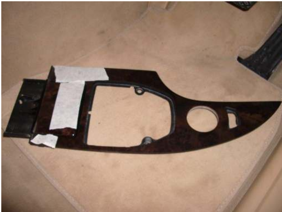
19. 2 screws holding wood trim down under gear surround (TIS says 3 but only 2 on my car). I believe the LCI (2007 onwards) has 2 extra screws at the front.
