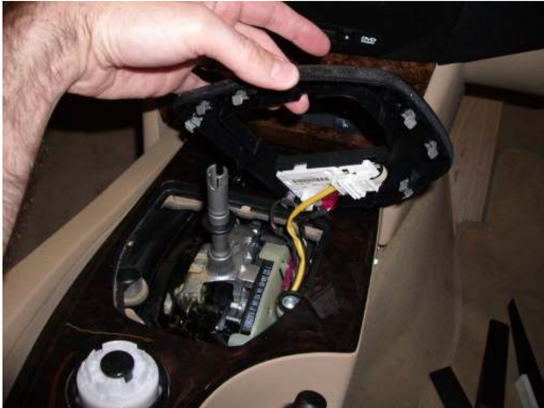
19. 2 screws holding wood trim down under gear surround (TIS says 3 but only 2 on my car). I believe the LCI (2007 onwards) has 2 extra screws at the front.
